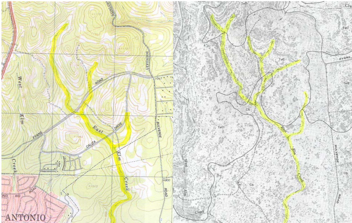
Figure 17. The stream network on USGS topographic maps (left) is often less detailed than on local soil surveys (right)
